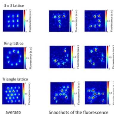
Single neutral atoms trapped individually in optical microtraps are incredibly useful tools for studying quantum physics, as the atoms then exist in complete isolation from the environment. Arrays of optical microtraps containing single atoms could enable quantum logic devices, quantum information processing, and quantum simulation.
