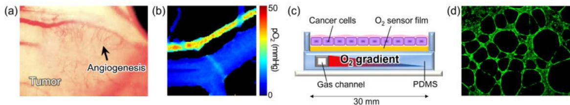
Figures (a) A microscopic image of tumor growth and angiogenesis, (b) laser-assisted  $pO_2$  imaging *in vivo*, (c) a schema of the microfluidic device with oxygen gradient and (d) a vascular network formed in the device.
