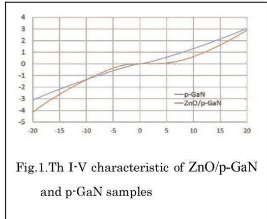
Fig.1. The I-V characteristic of ZnO/p-GaN and p-GaN samples
