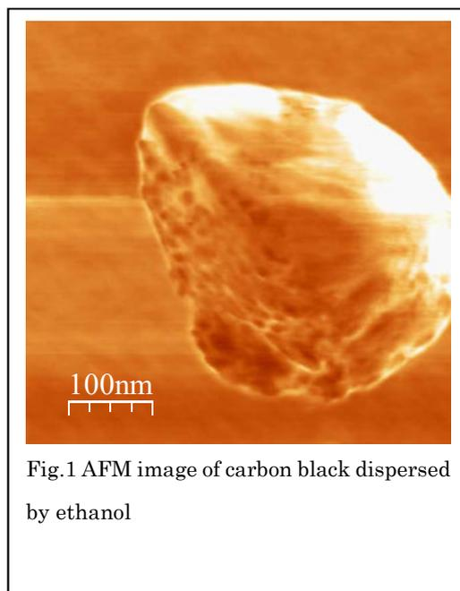
Fig.1 AFM image of carbon black dispersed by ethanol
