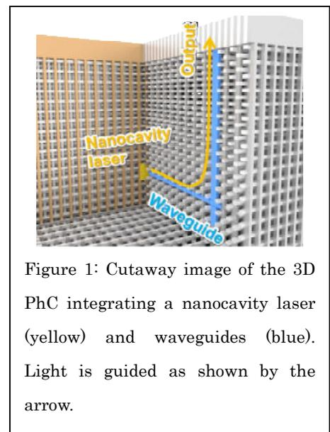
Figure 1: Cutaway image of the 3D PhC integrating a nanocavity laser (yellow) and waveguides (blue). Light is guided as shown by the arrow.
