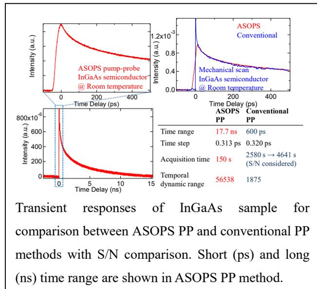
Transient responses of InGaAs sample for comparison between ASOPS PP and conventional PP methods with S/N comparison. Short (ps) and long (ns) time range are shown in ASOPS PP method.
