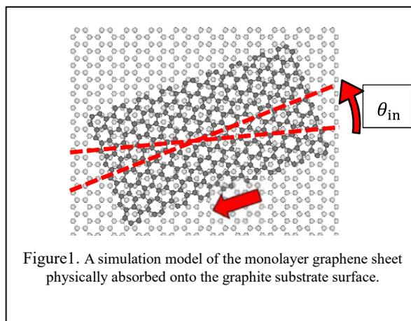
Figure1. A simulation model of the monolayer graphene sheet physically absorbed onto the graphite substrate surface.
