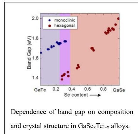
alloys the addition of selenium to the monoclinic  $\text{GaTe}$ -structure results in the linear increase of the band gap energy from 1.65 eV ( $m$ - $\text{GaTe}$ ) to 1.77 eV ( $x = 0.32$ ). Meanwhile the addition of  $\text{Te}$  to the hexagonal  $\text{GaSe}$ -structure results in a bowing trend for the band gap reducing it from 2.01 eV ( $h$ - $\text{GaSe}$ ) to 1.45 eV ( $h$ - $\text{GaTe}$ ).
