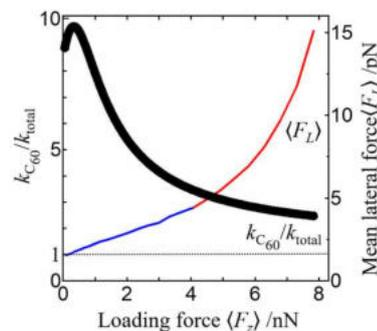
Fig.3 Ratio of stiffness of C<sub>60</sub> molecule to that of interface between C<sub>60</sub> molecule and graphene
