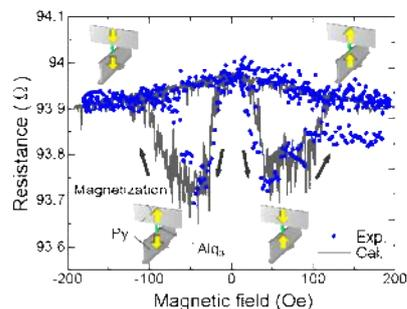
Fig. 1 MR effect of Py/ $\text{Alq}_3$ /Py at room temperature.
