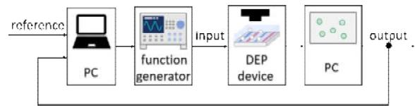
Fig. 1 Conceptual diagram of position feedback control system
