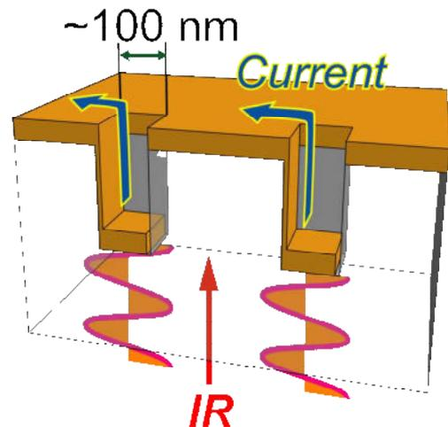
Fig. 1 SPR based photodetector
