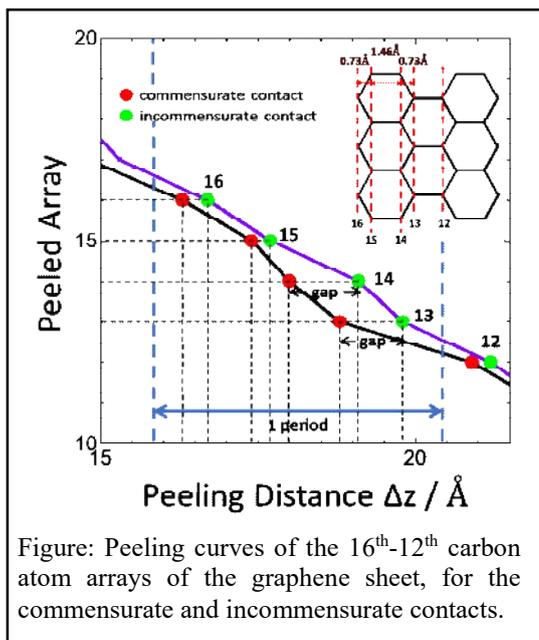
Figure: Peeling curves of the 16<sup>th</sup>-12<sup>th</sup> carbon atom arrays of the graphene sheet, for the commensurate and incommensurate contacts.
