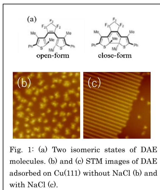
Fig. 1: (a) Two isomeric states of DAE molecules. (b) and (c) STM images of DAE adsorbed on Cu(111) without NaCl (b) and with NaCl (c).
