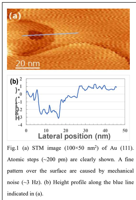
Fig.1 (a) STM image ( $100 \times 50 \text{ nm}^2$ ) of Au (111). Atomic steps ( $\sim 200$  pm) are clearly shown. A fine pattern over the surface are caused by mechanical noise ( $\sim 3$  Hz). (b) Height profile along the blue line indicated in (a).
