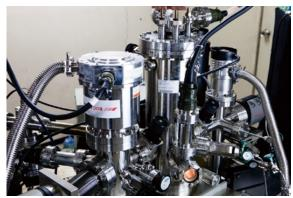
CoBIT (compact low-energy electron beam ion trap)
