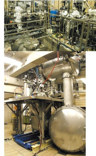
Tokyo-EBIT (high-energy electron beam ion trap)
