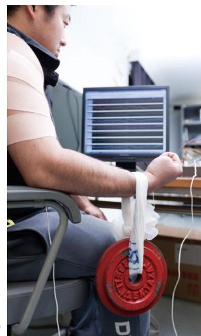
Wave propagation analysis system for electromyogram (EMG)
