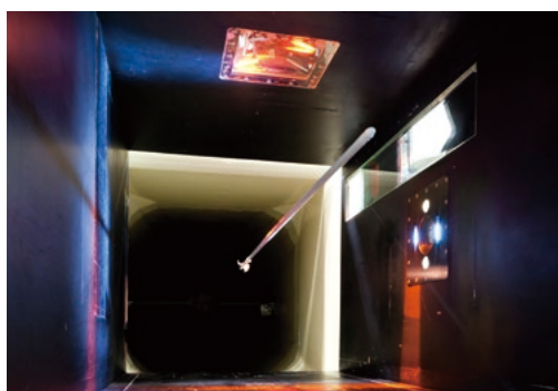
Internal view of wind tunnel experiment involving a magnetic suspension and balance system
