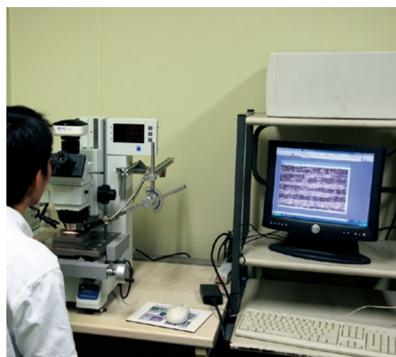
Image processing to evaluate cutting surfaces
