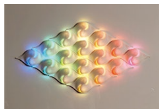
Figure 7: Three-dimensional tiles with built-in LEDs. The colors are controlled wirelessly.
