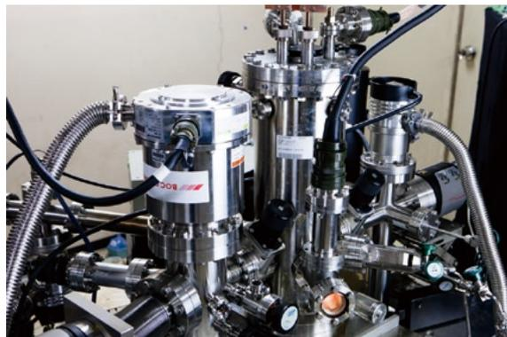
CoBIT (compact low-energy electron beam ion trap)
