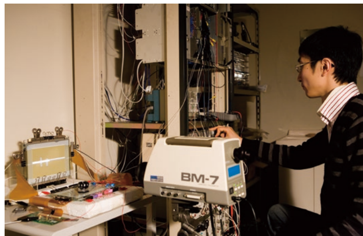
Measurement of the brightness of a small test PDP
